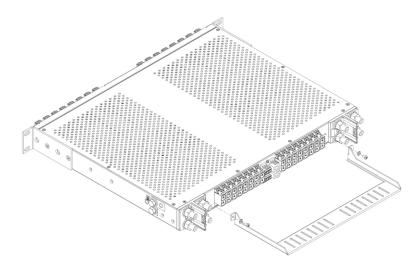
Fig. 2-4: Installing Optional -SC Tie Bar
