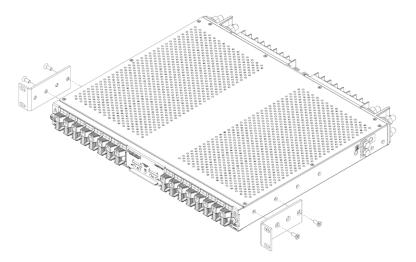
Fig. 2-1: Installing Mounting Brackets
