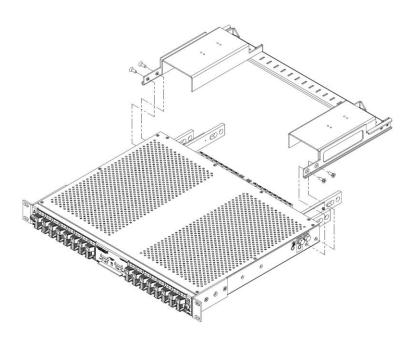
Fig. 2-2: Installing -C Tie Bar
