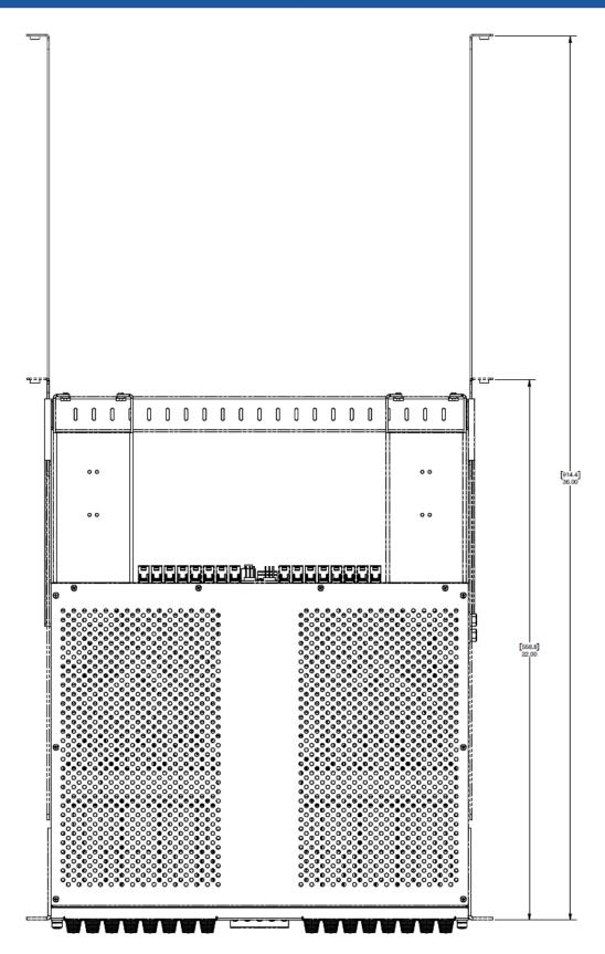
Fig. 3-15: Optional 4 Post Mounting Bracket (-C Versions)
