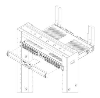
Fig. 2-8: Removing the Front Cover
