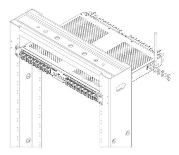
Fig. 2-6: Grounding Lug Connection
