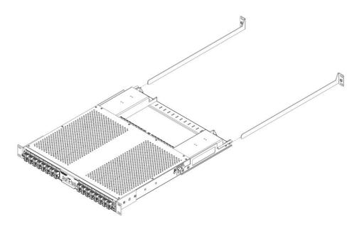
Fig. 2-3: Installing Optional 4 Post Mounting Brackets
