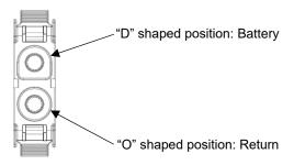
Fig. 2-18: Connector Front View
