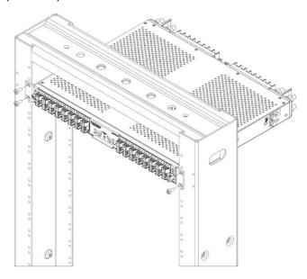
Fig. 2-5: Installing Panel in Rack
