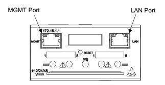
Fig. 2-15: CTRL Panel Connectivity Ports
