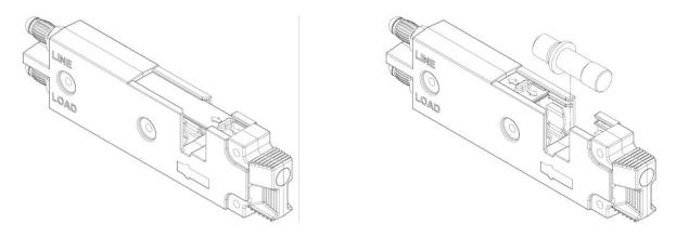
Fig. 2-12: Installing Fuse
