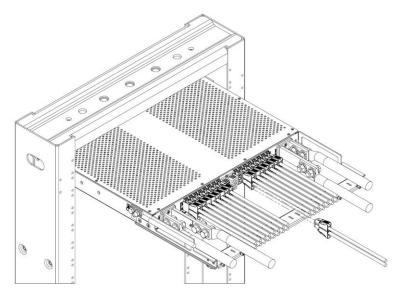
Fig. 2-20: Insert Connector
