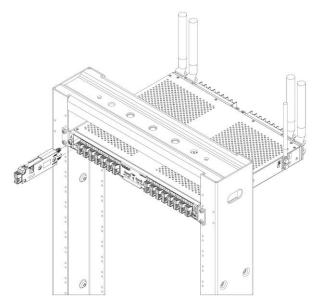
Fig. 2-11: Remove Fuse Holder
