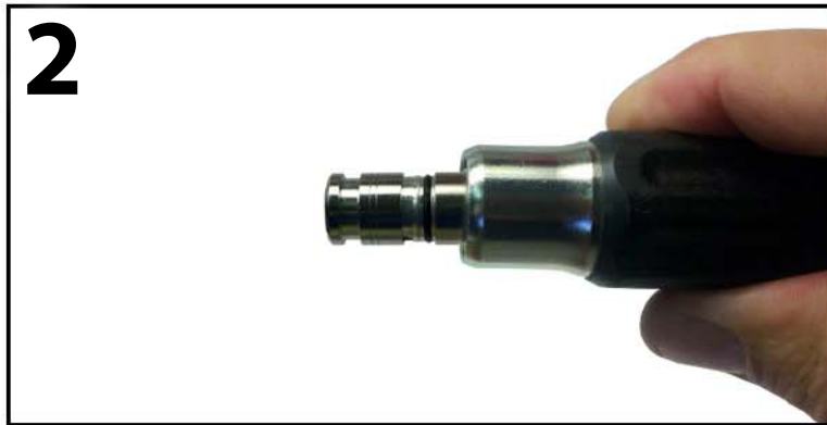
Insert the RCA connector into the large end of the tool
