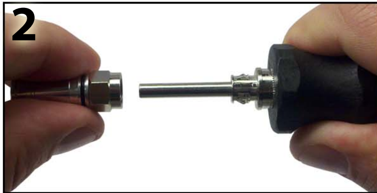
2 Insert the F connector onto the small end of the tool
