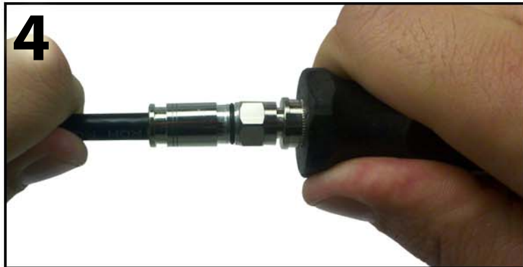
4 Firmly press the cable, ensuring the connector is inserted entirely
