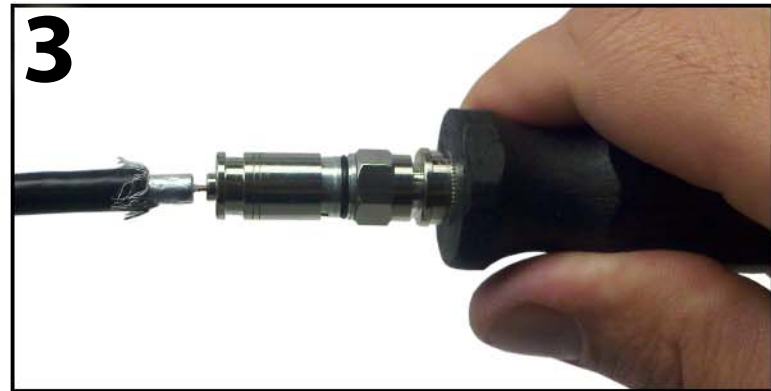
Guide your stripped coax into the end of the small tube on tool (This tube will guide your center conductor safely through connector)
